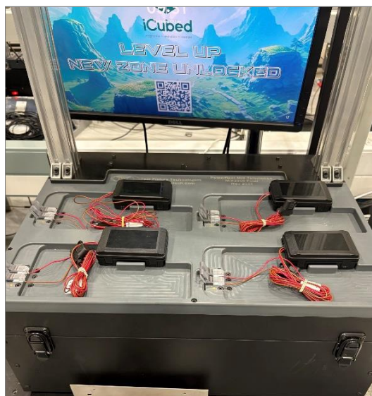
[D] MiX 2000 MK4 Final Test Bed-of-Nails
